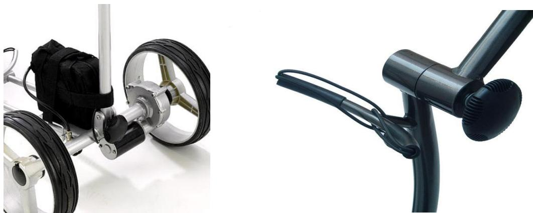
4. Place the battery pack (**F**) on the battery tray (**G**) and fasten the hook and eye strap (**H**) around the battery and fasten it tightly. Ensure that the power switch on the caddy handle is off. Insert the battery plug (**I**) into the golf buggy's outlet (**J**).
